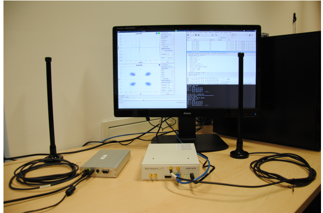
Figure 1: Overview of the demonstration setup. While the GNU Radio receiver is decoding WiFi frames, visitors can interact with the setup by grabbing one of the dipole antennas, move them around, and watch the impact live on the graphical outputs.
