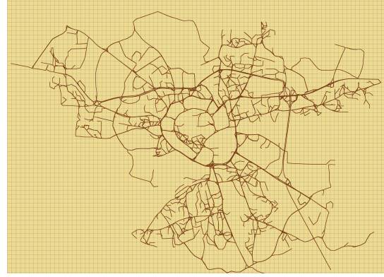
(b) Grid based approximation of the road map as contained in one vehicle's knowledge-base using the self-generation approach, 10 min into the simulation
