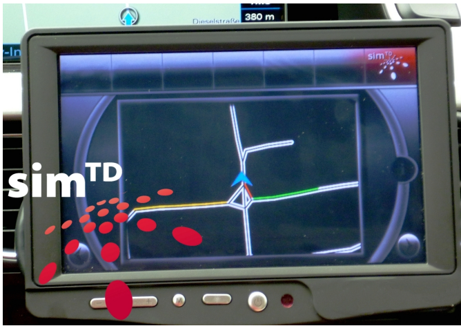
Figure 1. Photograph of a prototype of the simTD TIS in the field. Visualized is the knowledge-base (white) and stored traffic information: travel time measurements are indicated by colors.
