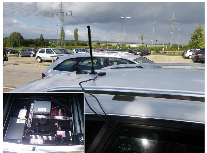
Fig. 2: Position of the shark fin antenna assembly, omnidirectional antenna, and GPS receiver on the roof; installation of the DENSO WSU 802.11p radio in the trunk (inset).
