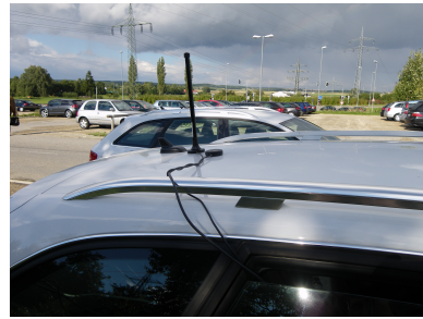
Figure 2: Position of the omnidirectional antenna and GPS receiver on the roofs of the cars.
